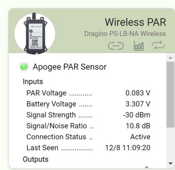
**Monitor Cards:** These cards display essential environmental parameters, including DLI, allowing users to monitor conditions at a glance.
